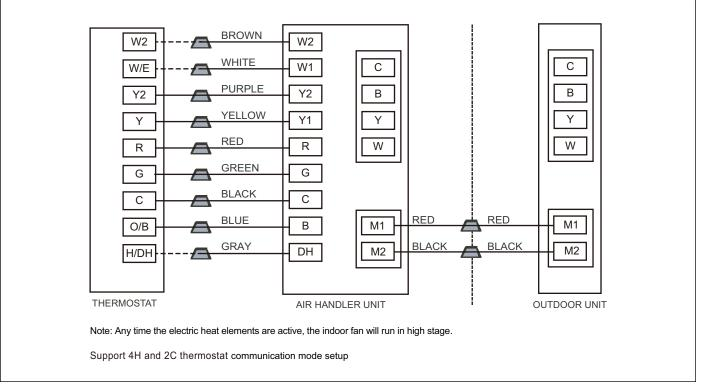
Figure 35 Control wiring for HP systems
