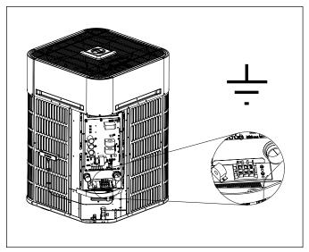
Figure 52 High voltage ground
