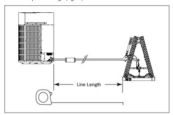
Figure 15 Required refrigerant line length
