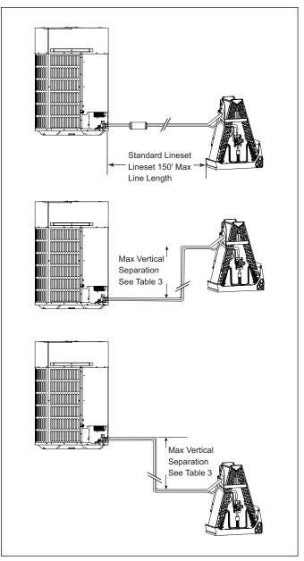
Figure 4 Refrigerant piping limits
