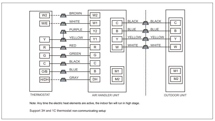
Figure 46 Control wiring for HP systems
