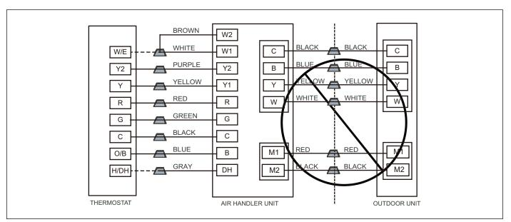
Figure 50 Incorrect wiring example
