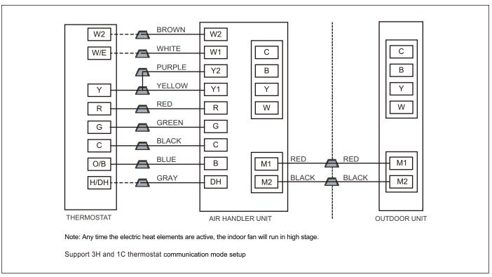
Figure 36 Control wiring for HP systems
