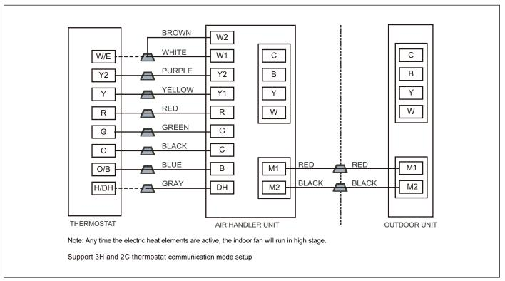
Figure 34 Control wiring for HP systems
