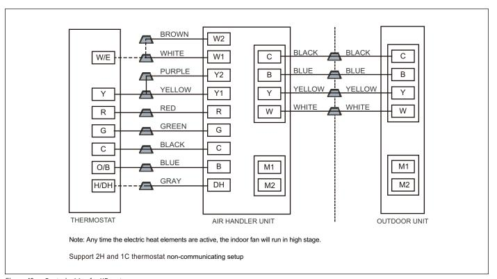
Figure 49 Control wiring for HP systems
