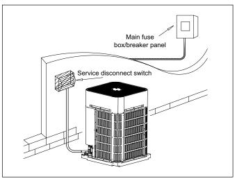
Figure 51 High voltage disconnect switch
