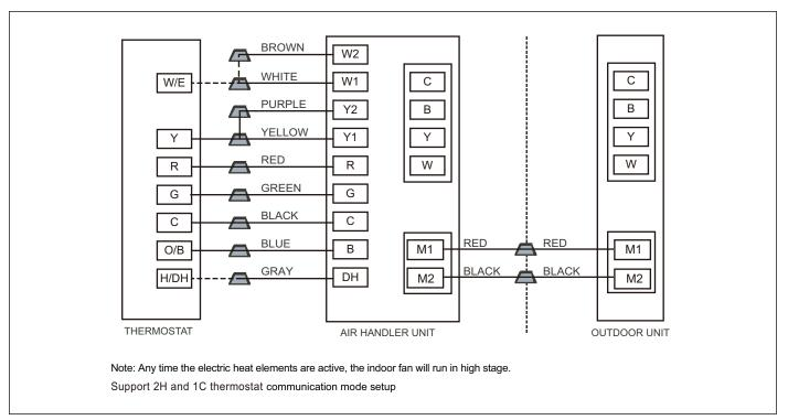
Figure 39 Control wiring for HP systems
