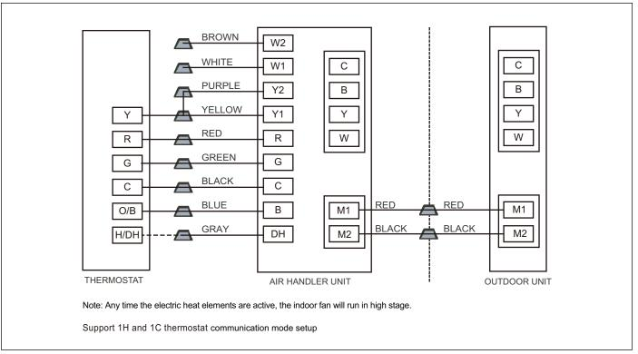
Figure 38 Control wiring for HP systems
