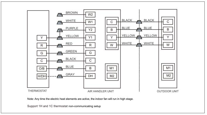
Figure 48 Control wiring for HP systems
