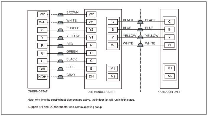
Figure 45 Control wiring for HP systems
