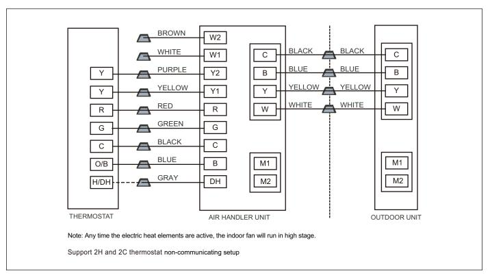
Figure 47 Control wiring for HP systems
