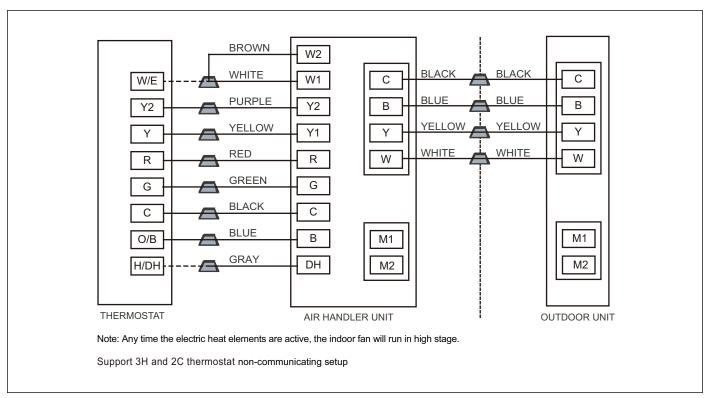
Figure 44 Control wiring for HP systems
