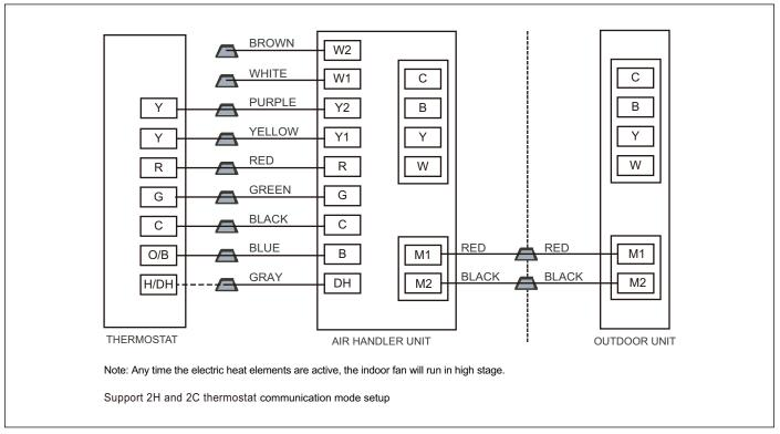
Figure 37 Control wiring for HP systems
