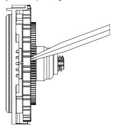
The drive cap assembly contains the drive cap, the main drive gear, drive cap spline, piston rod and various other parts that should not be dissembled in the field. The only replaceable part on the drive cap assembly is the o-ring. Attached to the drive cap assembly is the main piston (and a regenerant piston for 7-LXCTAIR, 7-LXIMAIR, 7-LXKATAIR, and 7-LXKATAIRO3 models).
