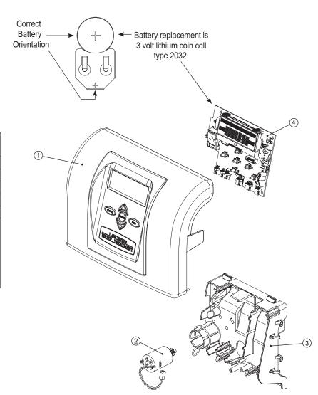
After completing any valve maintenance involving the drive assembly or the drive cap assembly and pistons, unplug power source jack from the printed circuit board (black wire) and plug back in or press and hold next and seconds. This resets the electronics and establishes the service piston position. The display should flash the software version and then reset the valve to the service position.
