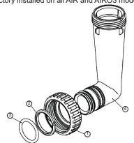
Do not use pipe dope or other sealants on threads. Teflon tape must be used on threads of 1" NPT connection. Teflon tape is not necessary on the nut connection nor caps because of o-ring seals.
