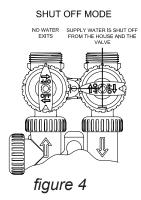
The working parts of the bypass valve are the rotor assemblies that are contained under the bypass valve caps. Before working on the rotors, make sure the system is depressurized. Turn the red arrow shaped handles towards the center of the bypass valve and back several times to ensure rotor is turning freely.
