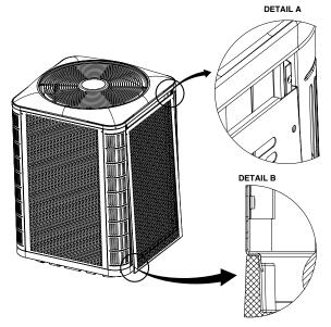
Figure 7. Panel Installation
