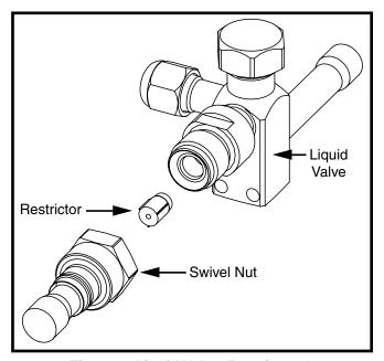
Figure 2. Liquid Valve, Restrictor, & Swivel Nut Adapter
