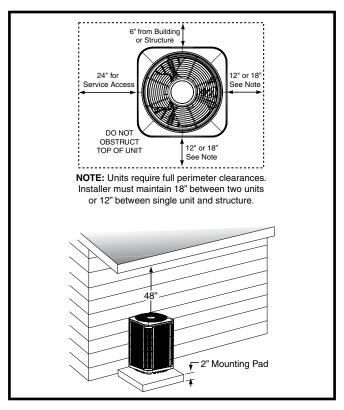
**Figure 1. Clearance Requirements**
