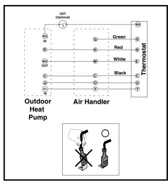
Figure 4. Typical Thermostat Connections
