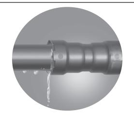
1 Identify an unpressed connection during pressure testing when water flows past the sealing element.
