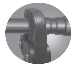
2 Upon identification, use the Viega MegaPress XL tool to press the fitting, making a reliable leak-proof connection.
