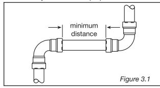
Minimum distance between two Viega MegaPress XL press connections 21/2" to 4"
