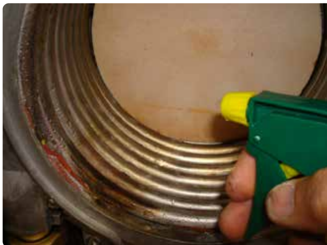
Figure 150 Cleaning the heat exchanger
