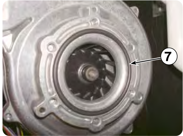
Figure 14 Insure "O" ring is in place
