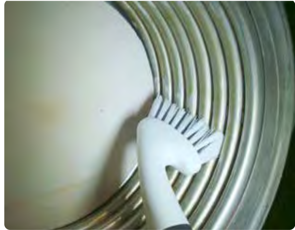
Figure 151 Cleaning the heat exchanger
