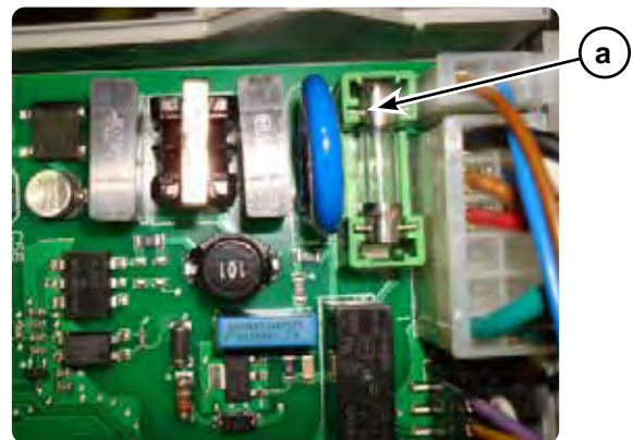
Figure 116 Thermostat-relay circuit fuse location
