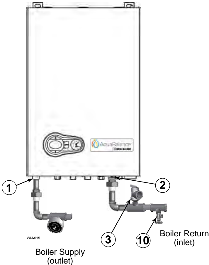
Figure 5 Install pipe fittings for relief valve and pressure/temperature gauge — DO NOT mount relief valve until AFTER hydrostatic testing (see legend below) ( Combi boiler shown )
