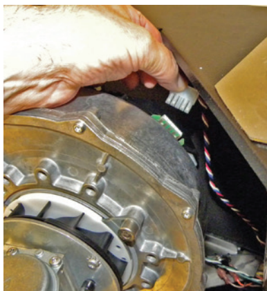
Unplugging fan control harness plug will drive the fan into manual high speed operation for vent leak test
