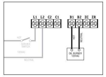
**STEP 2** Connect the burner circuit to **B1-B2**. (B2 is neutral.)
