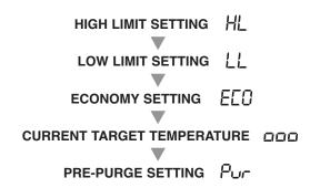
The display will return to boiler temperature (default) if Test/Settings Button in not pressed for 5 seconds.
