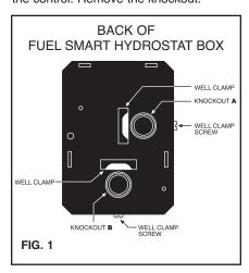
**STEP 2** Place control on the well. While holding box against well nut, tighten well clamp screw. (Fig. 2)
