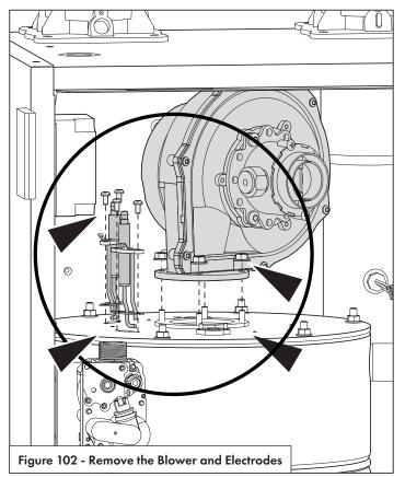
6. Remove the six (6) lock nuts securing the top plate to the heat exchanger. Remove the top plate and burner.
