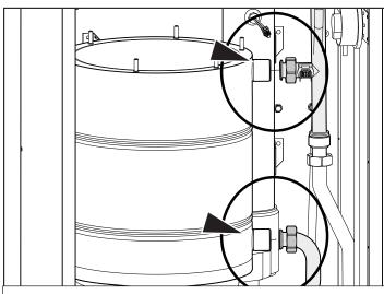
Figure 109 - Remove the CH Supply and Return Pipes
