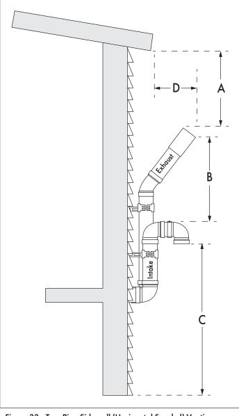
Figure 33 - Two Pipe Sidewall (Horizontal Snorkel) Venting
