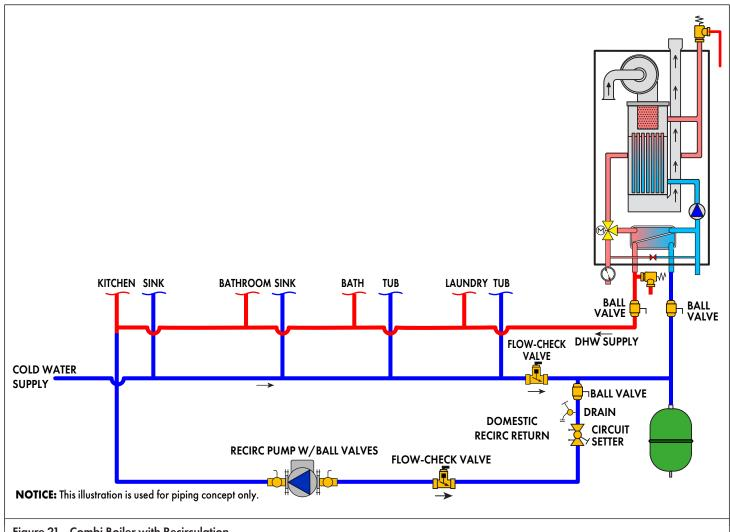
Figure 21 - Combi Boiler with Recirculation
