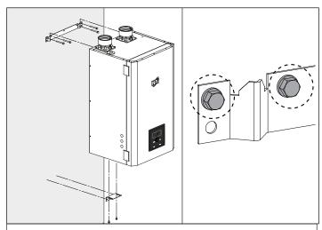
Figure 5 - Mounting to a Concrete Wall
