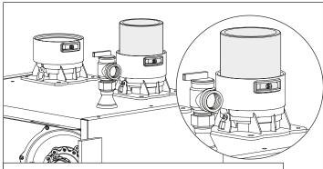
Figure 23 - Correct Installation into the Appliance Collar
