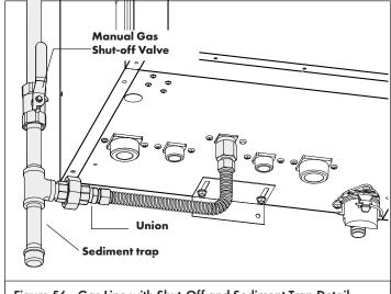
Figure 56 - Gas Line with Shut-Off and Sediment Trap Detail
