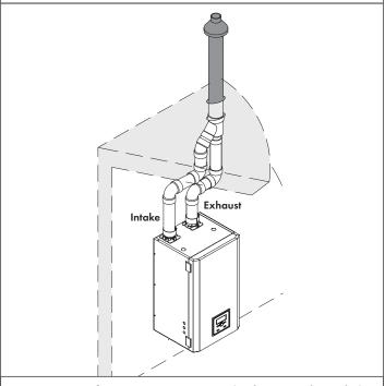
Figure 38 - Roof Concentric Termination (with Optional IPEX kit)
