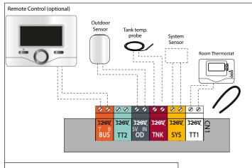
Figure 52 - Low Voltage Wiring Connections
