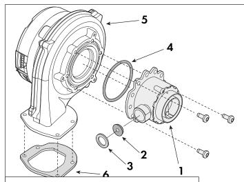
Figure 107 - Removed Fan, Mixer, and Components
