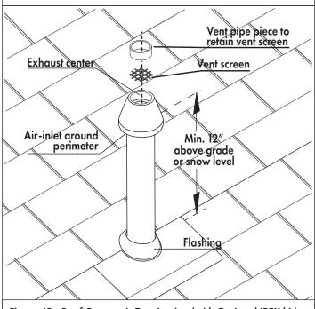
Figure 42 - Roof Concentric Termination (with Optional IPEX kit)
