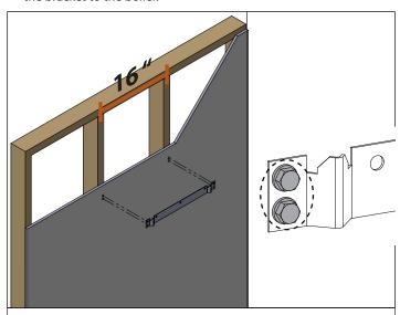
Figure 6 - Mounting the Bracket on 16" Center Studs
