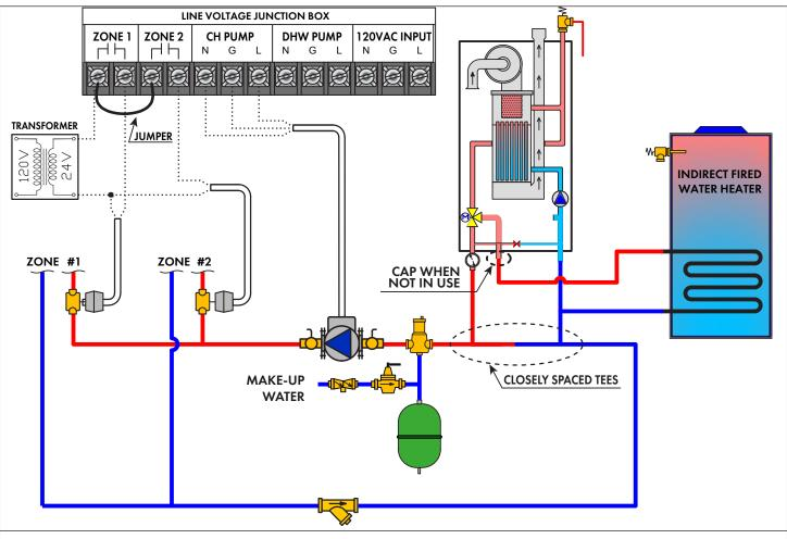
Figure 15 - Boiler with Single Central Heating Circulator
