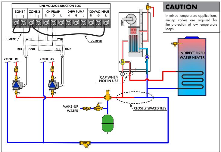
Figure 17 - Boiler with Multiple Central Heating Circulators
