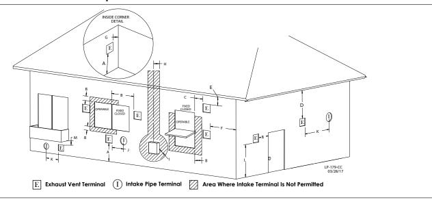
Figure 22 - Exit Terminals for Direct Vent Systems - ANSI Z223.1 / NFPA 54 for US and CAN/CSA B149.1 for Canada
