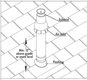
Figure 43 - Roof Concentric Termination
