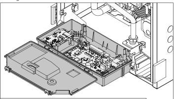
Figure 51 - Access to Low Voltage Wiring Connections
