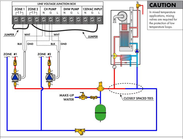
Figure 20 - Combi Boiler with Multiple Central Heating Circulators
