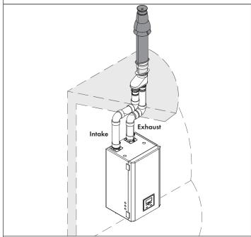
Figure 39 - Roof Concentric Termination (with Optional Duravent / InnoFlue Kit)
