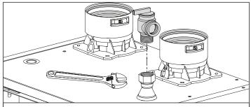
Figure 12 - Connect CH Pressure Relief Valve
