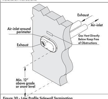
Figure 30 - Low Profile Sidewall Termination (with Optional IPEX Kit)
