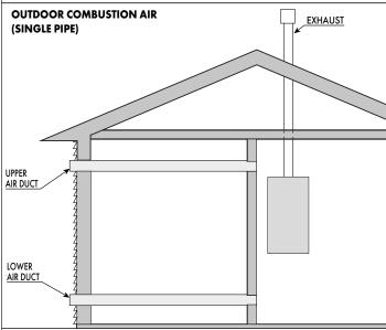
Figure 46 - Indoor and Outdoor Combustion Air - Single Pipe
