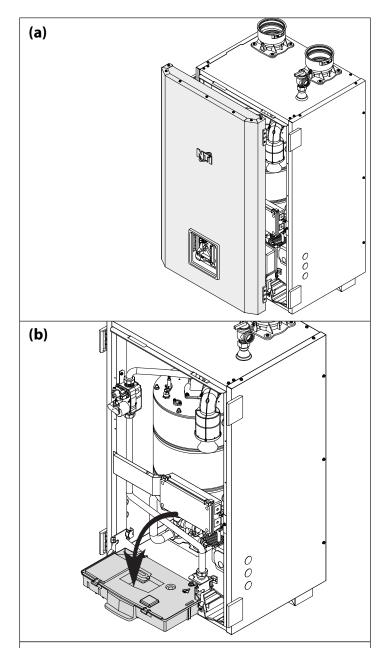
Figure 99 - Removing the Cover and Control Panel Housing
