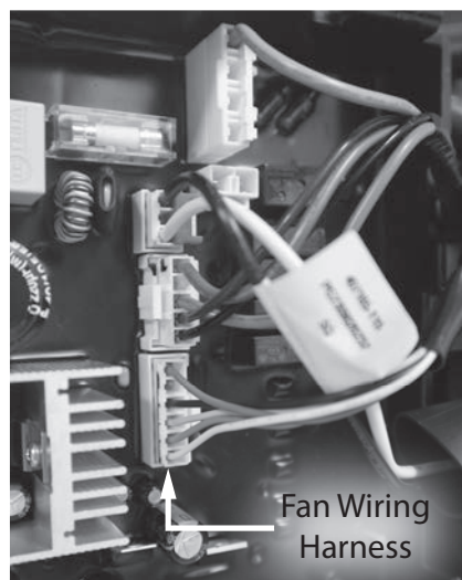
Figure 80 - Locate fan wiring harness on control board
