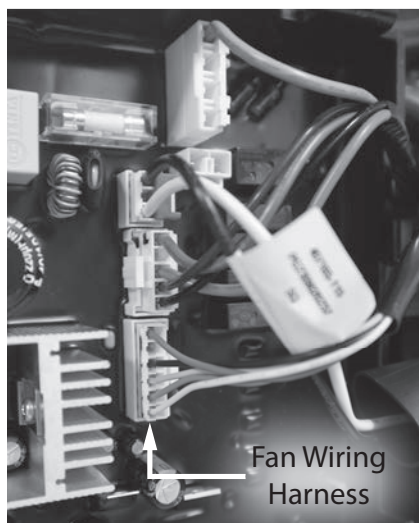
Figure 125 - Locate fan wiring harness on control board
