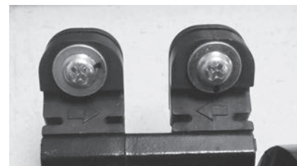
Figure 167 - Water pump gasket boot orientation
