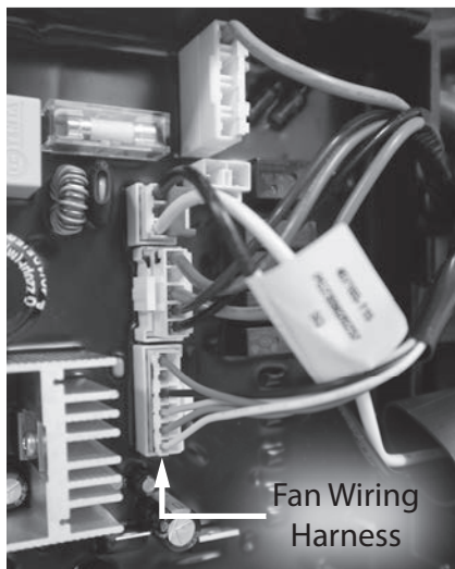
Figure 106 - Locate fan wiring harness on control board
