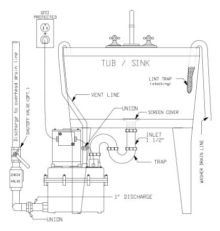
4. The installation of a shutoff valve is recommended in the discharge line.
