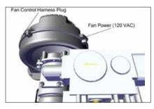
Figure 5B: 40-399 Fan control harness plug
