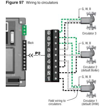
during DHW heating. To use factory default settings, make sure to connect the DHW circulator to terminals 1, 4 and 7, as below:
