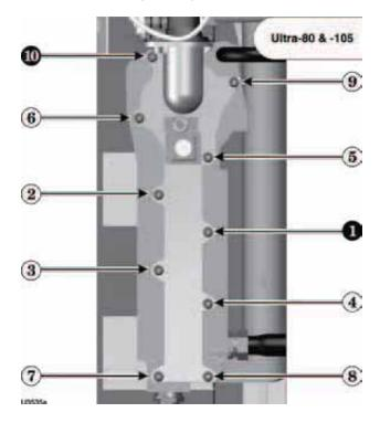
Figure 114 Cleaning the exchanger pin-side
