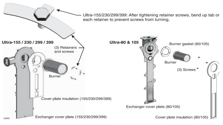
Figure 107 Burner assembly
