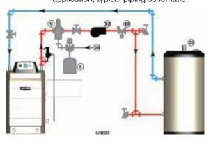
2. The PLUS water heater can also be installed as one of the zones in the system. This method, however, requires flow through the main system even during the summer (non-space heating) months. Piping as shown in Figure 9 and Figure 10, page 15 allows isolation of flow to just the water heater piping during non-heating periods.
