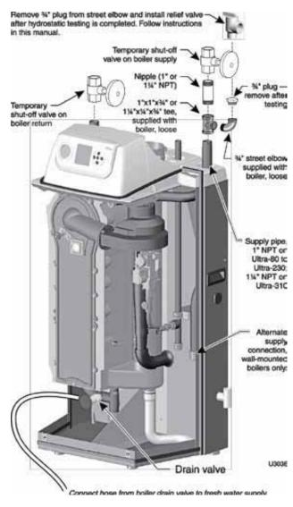
Do not use petroleum-based cleaning or sealing compounds in boiler system. Gaskets and seals in the system may be damaged. This can result in substantial property damage.
