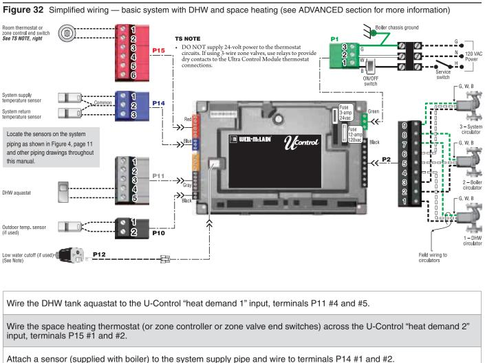
Attach a sensor (supplied with boiler) to the system return pipe and wire to terminals P14 #2 and #3. [Locate sensor in the position shown in piping diagrams on page 11 through page 15.]
