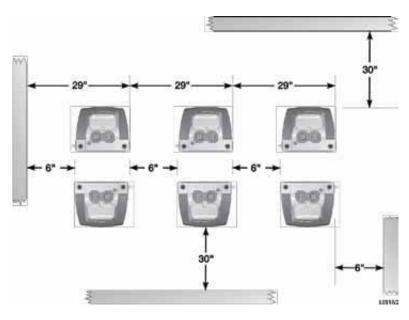
Figure 58 Wall mounting multiple Ultra boilers
