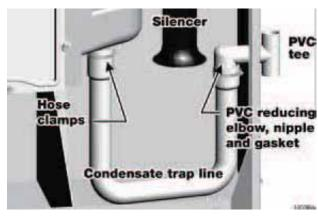
Figure 29 Condensate drain — Ultra-299 & -399
