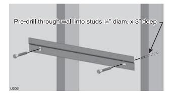
Figure 46 Place boiler on wall-mount bracket
