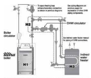
H1 = 0 (no DHW flow through boiler) H3 = Head loss through water heater H2 = Head loss through DHW piping U3046e
