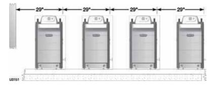
Figure 57 Back-to-back installation of multiple Ultra boilers
