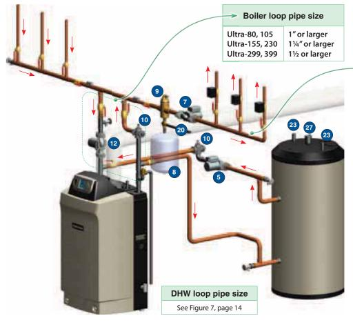
Figure 10 Ultra boiler with Ultra PLUS or PLUS water heater, typical piping schematics
