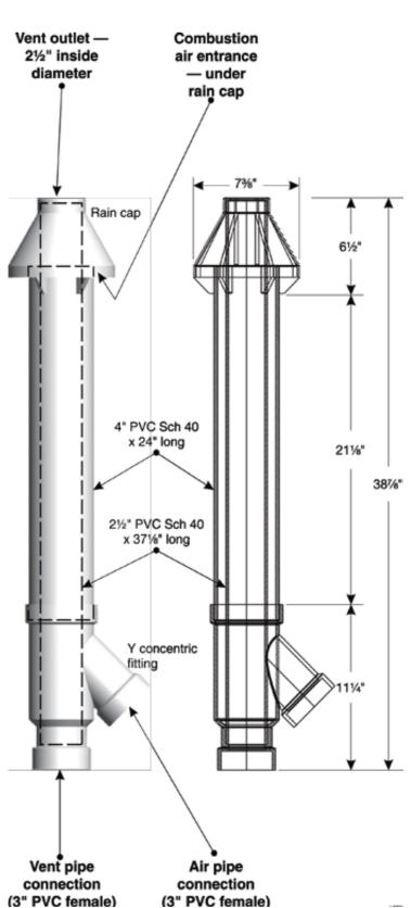
Figure 85 Weil-McLain 3" PVC concentric termination assembly
