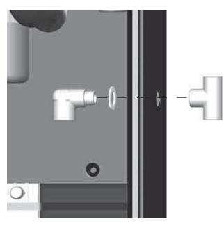
Figure 26 Condensate drain — Ultra-80 & -105
