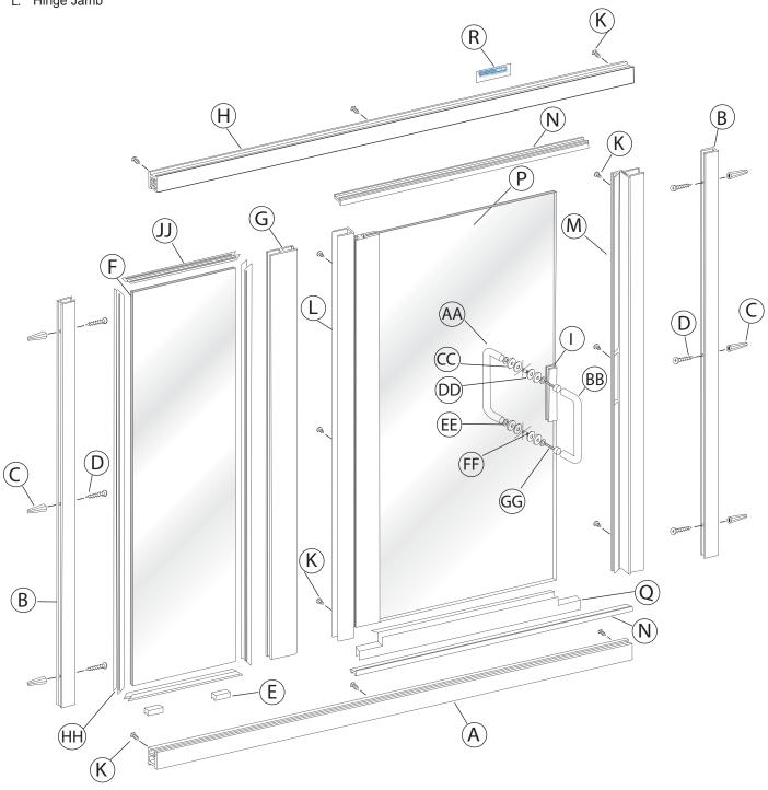
The BASCO 1413/1713 Continuous Hinge Shower Enclosure is completely reversible and may be installed swing-right or swing-left. The door may hinge from the wall or from the center-post. For maximum waterproofing, the hinge jamb should always be opposite the shower head. Using the illustration, determine the correct position for the door in your particular Infinity installation. This instruction sheet depicts a hinge-right installation.
