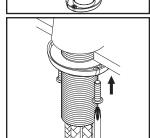
(2c) Thread locknut onto the faucet shank from underneath the sink. Position faucet to desired location from the top and handtighten locknut till it won't go further. Thread both screws on locknut and tighten screws on locknut with the help of a Phillips head screwdriver to secure faucet. (Note: Do not overtighten.)
