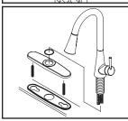
(3a) For 3-Hole Installation:- Thread mounting bolts to deck plate, apply plumbers putty under the base gasket, place faucet on the deck plate, make sure spout swivel angle are even to the right and to the left. Lead inlet & outlet flex hoses through center mounting hole to place faucet with deck plate and base gasket in position on the sink. Hand-tighten locknut to the faucet and tighten screws on locknut with the help of Phillips head screwdriver from underneath the sink.
