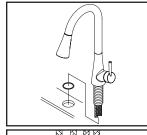
(2b) With flat side of the locknut facing down and the steel washer inside the locknut please follow the order as the drawing shows to insert flex hoses through the center hole of the
