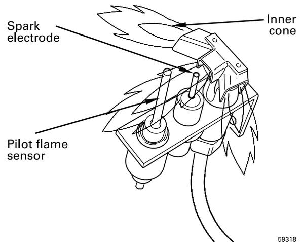
Figure 22 Typical main burner flame
