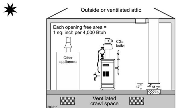
Figure 5 Air from outdoors – horizontal ducts
