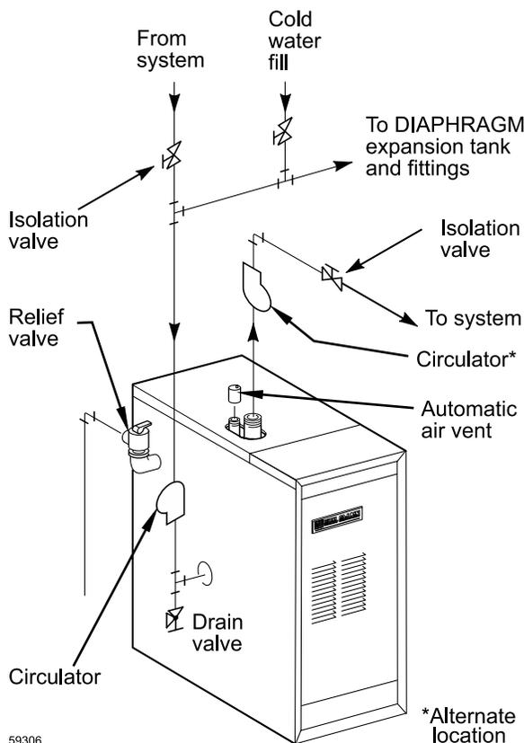
**Figure 10** Closed-type expansion tank — Single-zone system using closed-type expansion tank. See Table 3 for piping sizes.
