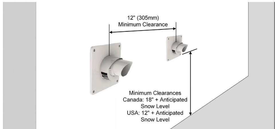
Figure 11a: Horizontal Concentric Termination - Two Kits
