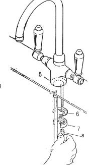
4. Under the sink, stack the half ring rubber gasket - 6, the half ring mounting plate - 7, then the mounting nut - 8 onto the stud.
