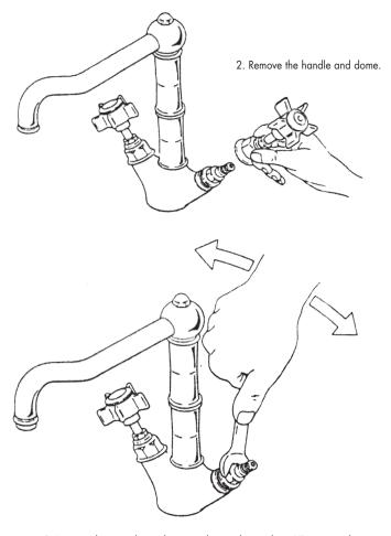
3. Remove the cartridge with a smooth jawed wrench or  $17 \mathrm{mm}$  wrench
