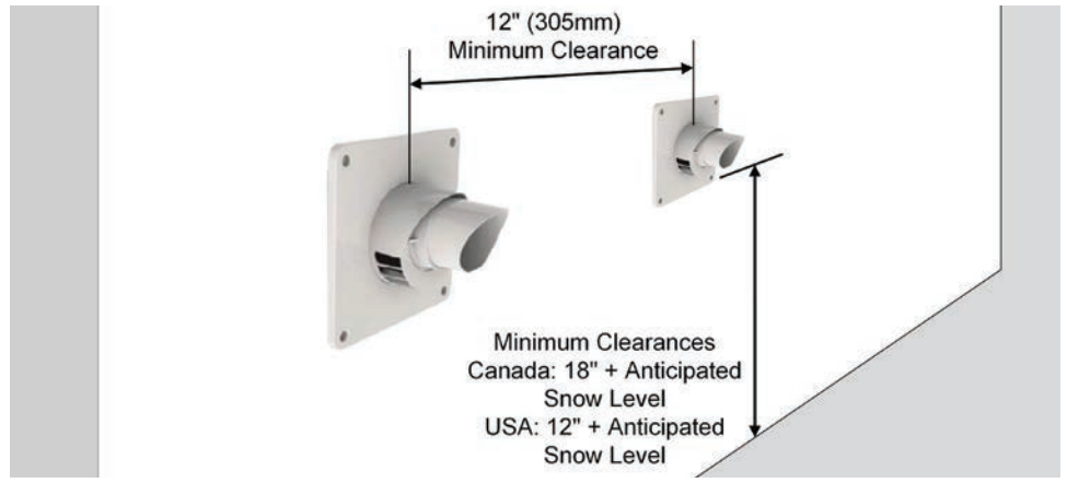
Figure 9a: Horizontal Concentric Termination - Two Kits
