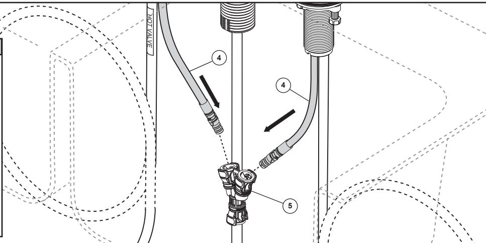
Insert faucet outlet tubes (4) into Y-shaped connector (5) until it clicks. Pull down moderately to ensure the connection has been made.
