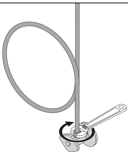
Secure nut to supply valve and hand tighten, then one additional turn with wrench. Do not over tighten. Repeat for other side. Do not use pipe dope or other sealants on water line connections.
