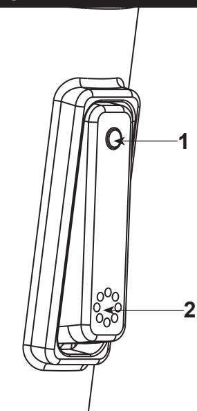
Sprayer will lock into position when brought into proximity of the spout magnet. The sprayer can be removed by either pulling directly out from the spout or by twisting 90° in either direction which will cause the magnets to repel and the head to decouple from the spout (recommended).
