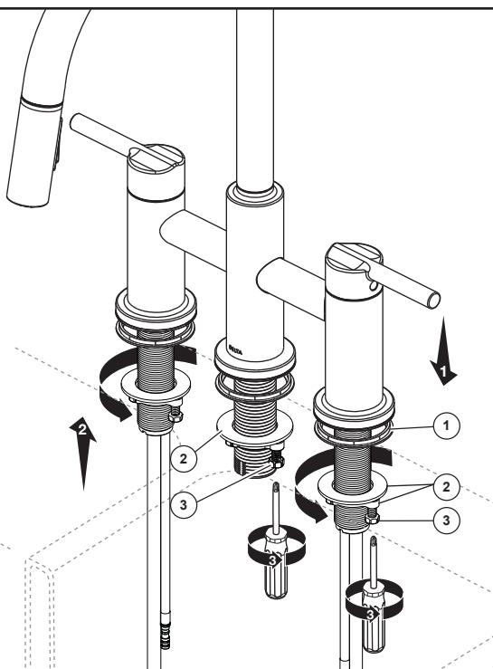
Install base plate (1). Secure spout and mounting shank with mounting nut and washer (2). After hand tightening mounting nut, tighten screws (3) with Phillips screwdriver until snug.
